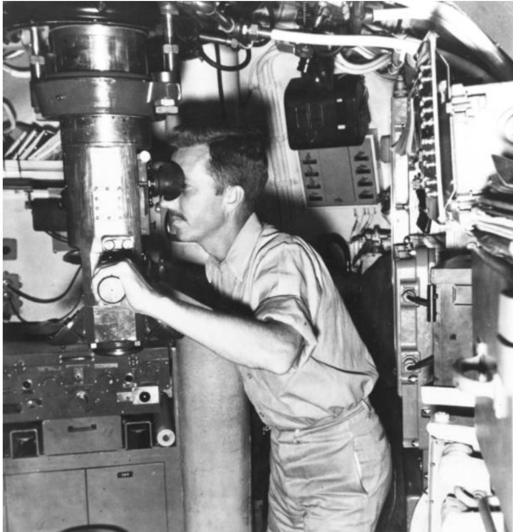
An officer aboard the submarine USS Bullhead looking through the aft periscope, about May 1945, location unknown.
